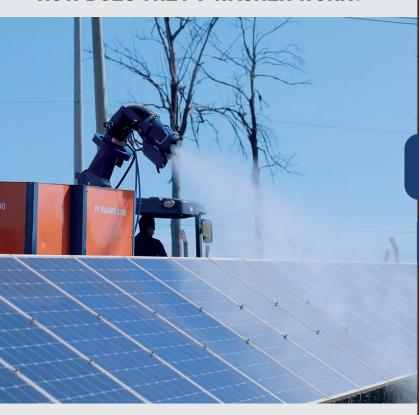
Carry out the cleaning of your ground panels by controlled air-jet spraying, utilizing only 1.2 liters of water per module, avoiding damages and preserving the warranty of the modules.
