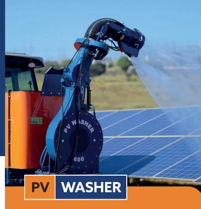
Clean your photovoltaic plant's modules without any loss in power generation.
